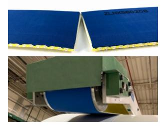
**MIR #1961591** replaces flat nylon core belting – requiring minimal downtime for installation with proven reliability and performance. With its spiral screen design, welding the belt endless is not required and there will be no mechanical lace.
